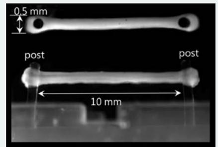
Advanced isometric force measurement system is capable of detecting more subtle effects on hvCTS function, as demonstrated here in a disease model with or without rescue.
